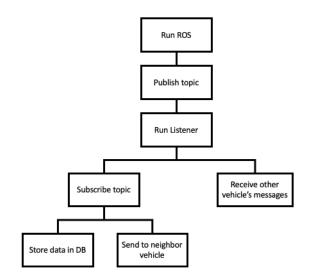
Fig. 3. Vehicular Web Client's work-flow diagram.
