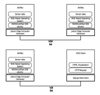
Fig. 2. A web-based system structure.
