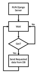
Fig. 4. Vehicular Django web server's work-flow.
