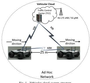
Fig. 1. Vehicular cloud system structure.
