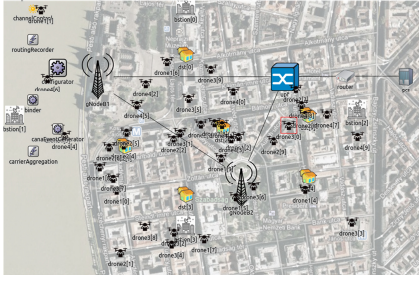
Fig. 3. A 5G-Enabled Network Simulation Scenario in OMNeT++.
